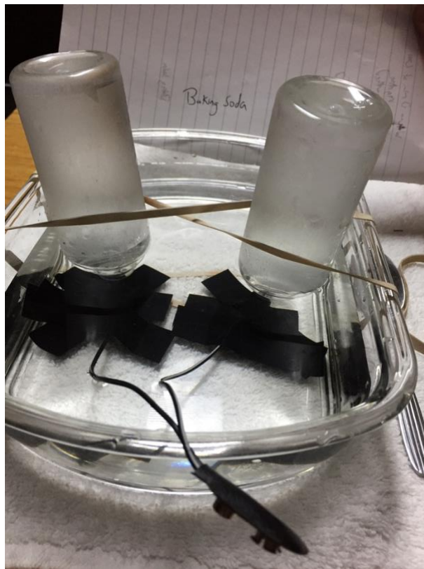
Figure 1: Electrolysis experiment setup with baking soda
